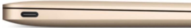
Figure 2: A single USB-C type connector indicates a MacBook with a USB 3 port. This is not a Thunderbolt port.
